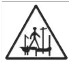
Danger Scaffolding Incomplete
